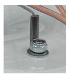
Please note that the bowl at the top of the parabola is caused by tightening the nut. It is necessary to tighten this nut over the entire length of the thread. As you can see, the blue brake must be screwed onto the threaded rod to prevent it from unscrewing. If this were not the case, the bowl would cause vibrations that would be detrimental to the sound of the speaker, or worse still, the spherical part would not be well maintained and could fall.
